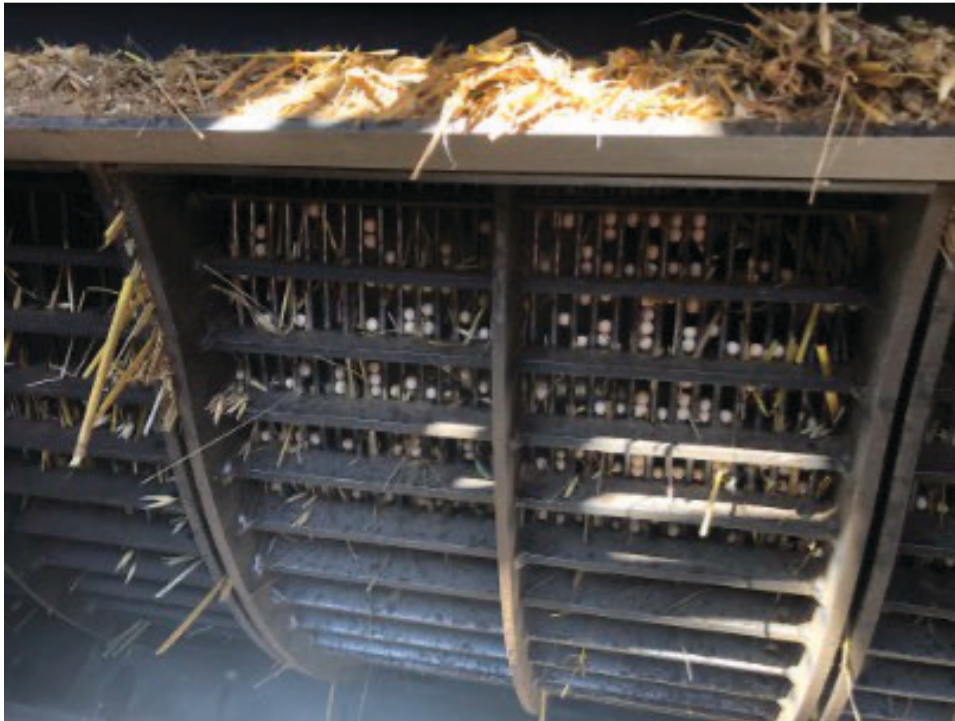
Photo: Oat-pea intercrop in combine concaves. Combining poses one of the most significant obstacles to raising a profitable oat-pea intercrop.
